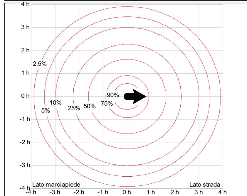
$$E \text{ (lux)} = \frac{E_{\text{max}} \times E\% \times F}{h^2 \times 1000}$$
